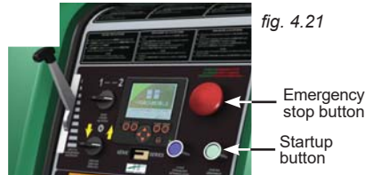
fig. 4.21 Note: The F2 Series control panel layout is the same for both gas-powered and electrical units; some controls, such as the choke button, are disabled for the electrical unit
