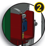
Gate detection switch located on the front gate assembly
