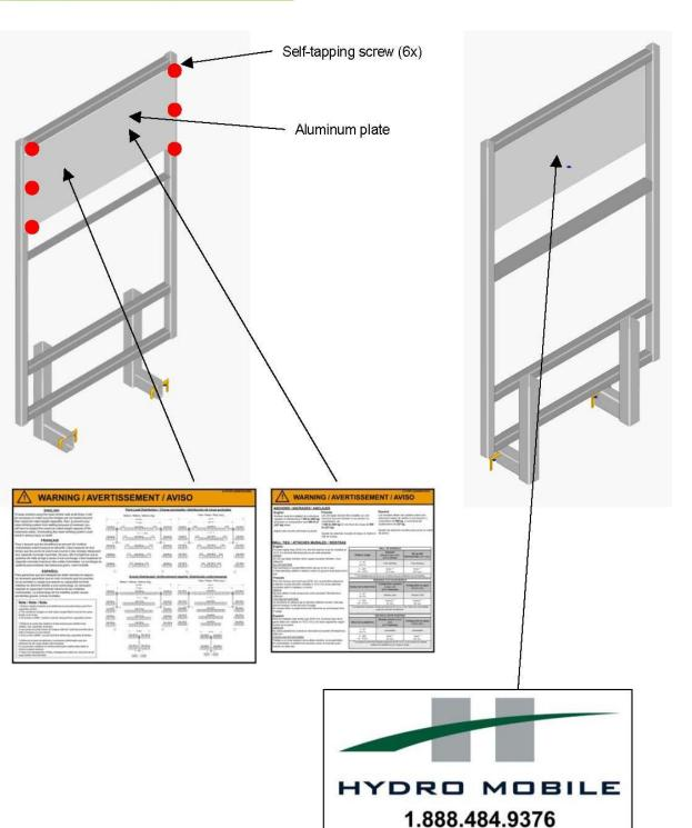
The Operator's manual casing attachment bracket will have to be mounted on the 4x2 rectangular tube as shown on the picture below with 4 self-taping screws. Then, use the clamp to fix the casing in place with Release 3.1 of the Operator's manual. On new units, please weld the attachment bracket as described in PIP-057 issued last April 22<sup>nd</sup> 2005 and add casing with Release 3.1 of the Operator's manual.
