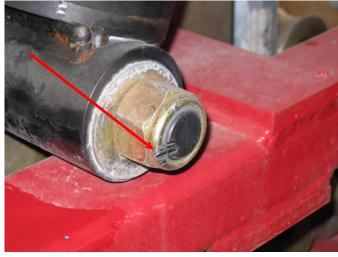
4. Unscrew the lower pivot from the brake box housing using a 1 1/2" wrench. If the nut turns and unscrews from the lower pivot shaft, repeat step #3. If step #3 is still unsuccessful, the nut will need to be welded to the shaft for removal. If welding is necessary, it is mandatory to remove the pressure transducer from the main hydraulic distribution block.
