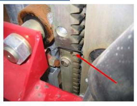
3. Punch the shaft and nut to lock the nut on the lower pivot shaft. Using a zip gun facilitates this step.
