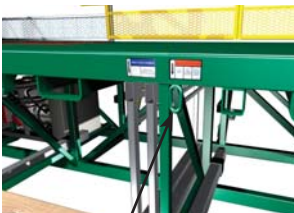
fig. 2.7 Tie point located at the front of the motorized unit
