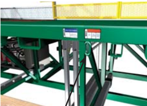
fig. 2.7 Tie point located at the front of the motorized unit
