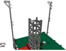
Diagonal brace of post facing toward face of work
