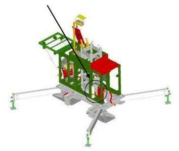
Position Toolbox bracket  $1\frac{1}{2}$ " from the bottom tube and fasten using 4 self tapping screw supplied.
