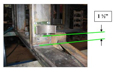
Install Toolbox tube on bracket using hose clamp
