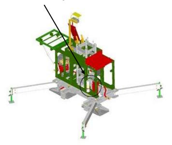
Position manual storage container bracket -11/2" from bottom tube and fasten using 4 self tapping screws supplied.
