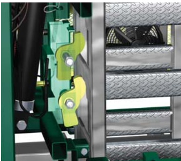
Safety hooks in normal working position
